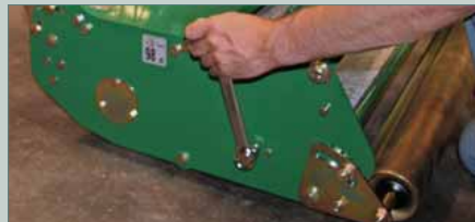
Tighten retaining bolt
