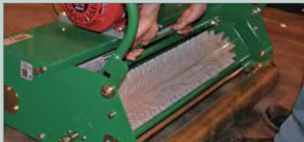
Lower cassette onto back tie bar and slide cassette across
