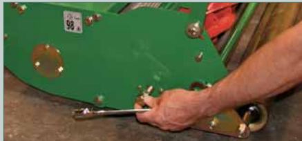
Loosen retaining bolt and slide cassette across
