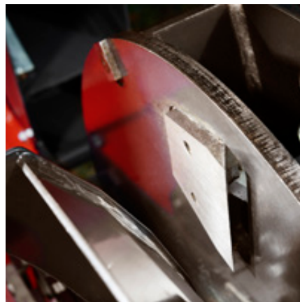
Displaced blades (2 pcs.) constantly engaging material
