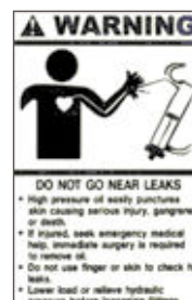
High oil pressure hazard
