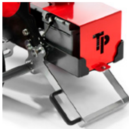
Foot brake stabilization
