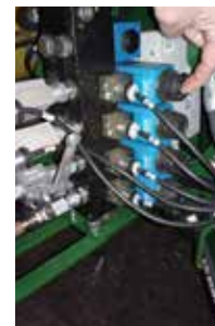
Figure C Button shown will make the wing go down. Button on the opposite side will raise the wing.
