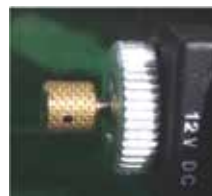
This shows the manual override position with the thread out. IMPORTANT - The check will not work in this position & this should be used for maintenance purposes only. Manual override should not be used when operating the machine normally.
