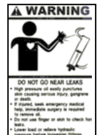
High oil pressure hazard
