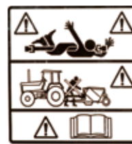
PTO entanglement hazard - keep clear of PTO drives.
