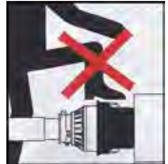
Do not use the shaft cone as a step
