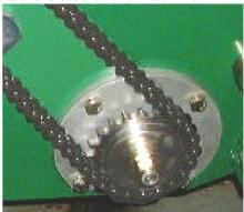
Take off the cutting cylinder drive chain and withdraw the cylinder sprocket (use 3 leg puller). Unscrew the four bolts securing the bearing housing on the main side plate (use 1/2" A/F spanner) and withdraw the housing (use 3 leg puller). Then unscrew the set screw on the left hand side of the cassette assembly (use 15/16 A/F spanner). The cutter cassette unit can now be moved fully to the left hand side of the machine and lifted out.
