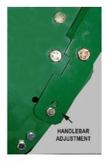
For operator comfort the handle bar must be adjusted using the various hole positions provided on the side plates of the machine (use 9/16" A/F/ spanner).
