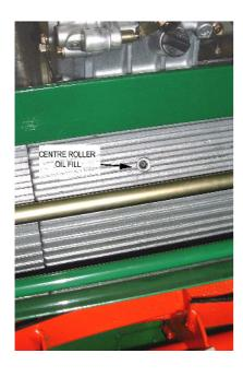
The main drive roller is split into three sections incorporating a differential gear system running in an oil bath. Every six months the old oil should be drained off and the bath replenished with clean oil (560cc) (1 pint).
