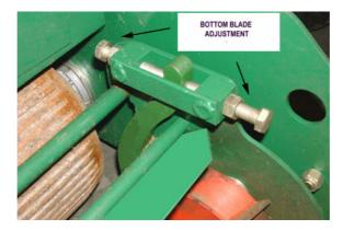
To adjust the shear blade, firstly slacken the four adjusting screws and locknuts positioned in opposed pairs at each end of the cutter cassette frame. Then move the shear blade to the cutting cylinder all along it's length and bring the screws up to the levers so that the position of the blade is maintained. Tighten the screws and locknuts.
