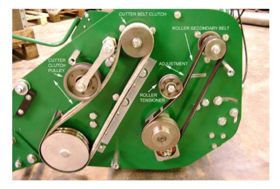
"Belts will be sufficiently tensioned if the deflection force applied at mid span to produce a deflection equal to 16mm per meter of span distance falls between 5 and 9 Newtons per Rib" (TBA Belting).
