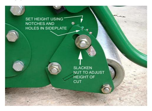
The length of grass after cutting, or depth of scarification / dethatching / brushing, depends on the setting of the front roller in relation to the main frame of the machine.
