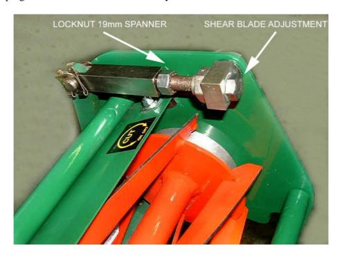
The adjustment is facilitated by turning the spring loaded bolts on either side of the cutter cassette in the direction indicated by the decals. The shear blade carrier is pivoted in the cassette sideplate and as the "ear" is moved back the blade gets closer to the cylinder. Adjust until both sides are just in contact with the cylinder. Do not tighten one side excessively as this will cause twist in the bottom blade.
