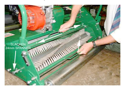
Undo the 5/8" UNF Bolt located on the right hand side of the machine on the centreline of the cutter shaft. Use the 24mm spanner provided
