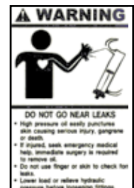
High oil pressure hazard
