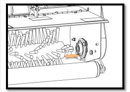
Raise the reel completely clear of the ground using the micro adjuster. Remove the nuts and washers (*on the right hand side of the machine*) that secure the bearing to the side plate. Slide the tine reel out of the socket on the stub shaft (*see image*). Lower it to the ground and remove it from the machine. Reverse the procedure to fit alternative reel.
