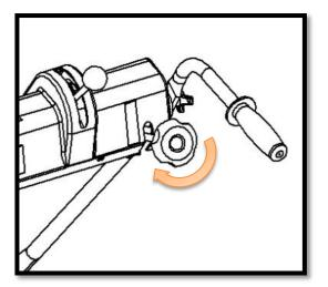
The blades must be **CLEAR** of the ground before adjustment commences. The depth of cut is adjusted by varying the height of the front rollers, using the micro adjuster. Start the engine and allow to warm up. Engage the ground wheel and reel drives and lower the reel using the micro adjuster until the required amount of thatch is being removed. Always disengage the reel drive when the machine is stationary on the green.
