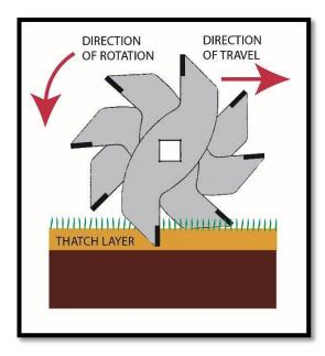
The Rotorake principle incorporates a series of blades rotating at high speed in the opposite direction to that of the conventional cylinder mower. The blades therefore cut upwards, continuously taking grass fibre away from the surface rather than pushing it into the surface of the turf. This also ensures that the machine is held to the ground and a regular working depth maintained.
