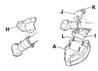
Remove the mounting plate (H). Fit the adapter (I) and bracket (J) with the two screws (K) as shown. Fit the blade guard (A) to the adapter using the 4 screws (L) as shown.
