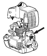
Some mufflers are equipped with a special spark arrestor mesh. If your machine has this type of muffler, you should clean the mesh at least once a week. This is best done with a wire brush.
