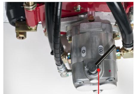
Reel Motor shut-off valve
